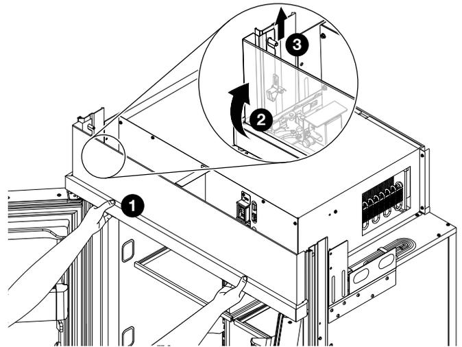
3. Remove the two side trims which support the grille from the refrigerator by unscrewing the six 1/4" hex screws. Save the screws and trims for assembly prior to installing the unit in the cabinetry.
