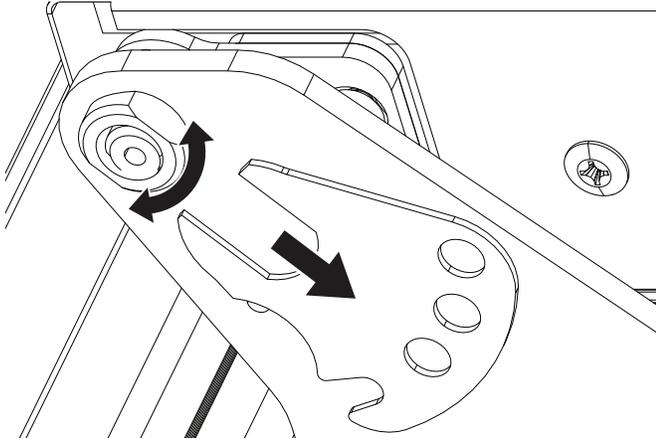
4. Turn the bushing located underneath the bottom of the hinge using a 1/2" open end wrench. Turning the bushing to the left will lower the door. Turning the bushing right will raise the door. See illustration.
