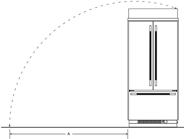
**NOTE:** Tipping Radius dimensions below are with upper grille and side trims removed.
