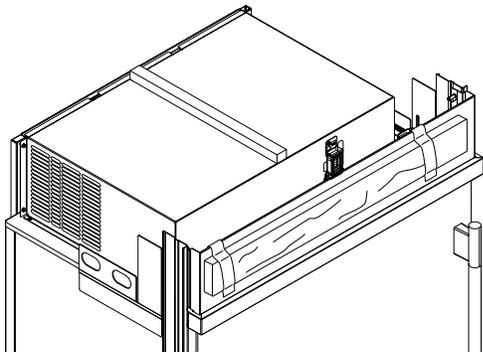
2. Remove the upper grille from the refrigerator. Save for final installation.
