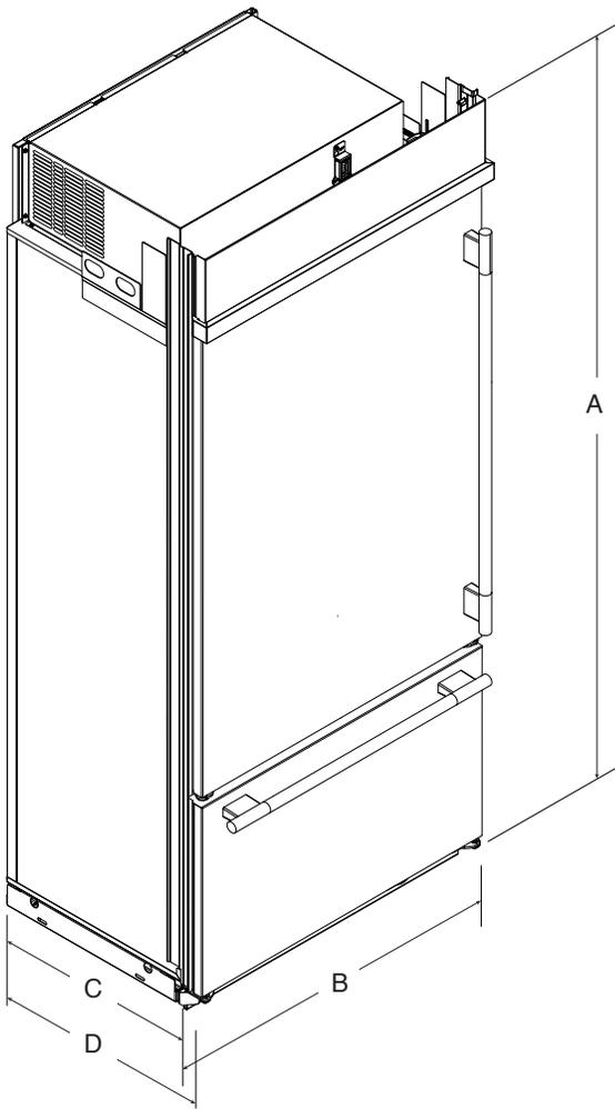
\*When leveling legs are fully extended to 1¼" (31.8 mm) below rollers, add 1⅞" (28.6 mm) to the height dimensions.
