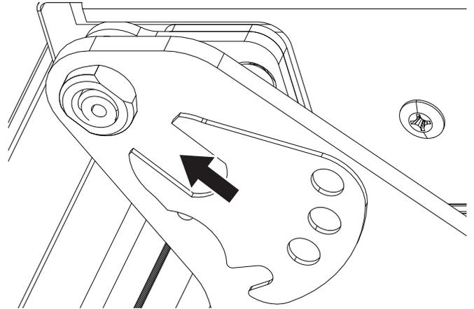
7. Turn the bushing slightly to align the hinge and locking plate screw holes.
