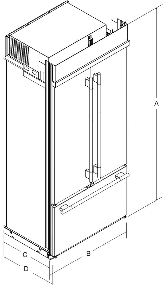
\*When leveling legs are fully extended to 1¼" (31.8 mm) below rollers, add 1⅞" (28.6 mm) to the height dimensions.
