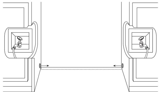
**IMPORTANT:** Route and tape the waterline along the wall, to prevent kinking during refrigerator placement.
