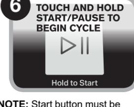
**NOTE:** Start button must be held for 1 second to start cycle. Once the bottom line of lights left of the Start button are illuminated, release the Start button.
