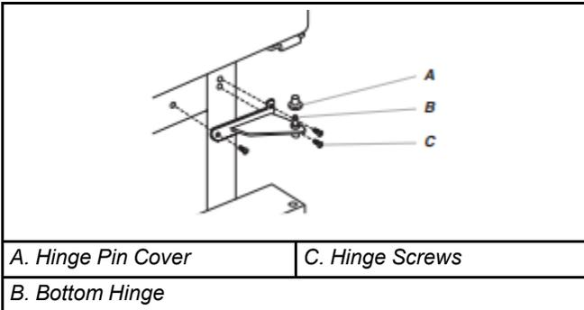
**NOTE:** Provide additional support for the refrigerator doors while the hinges are being moved. Do not depend on the door gasket magnets to hold the doors in place while you are working.
