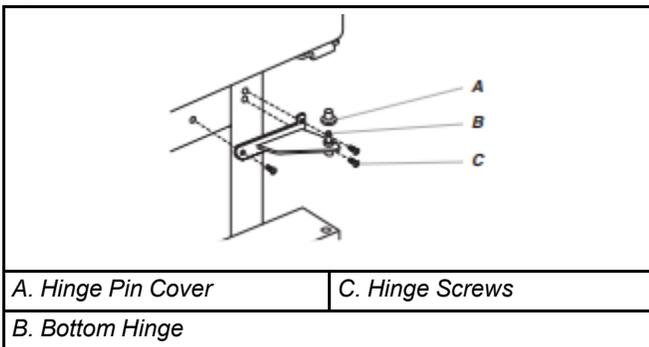
**NOTE:** Provide additional support for the door while the hinges are being moved. Do not depend on the door gasket magnets to hold the door in place while you are working.
