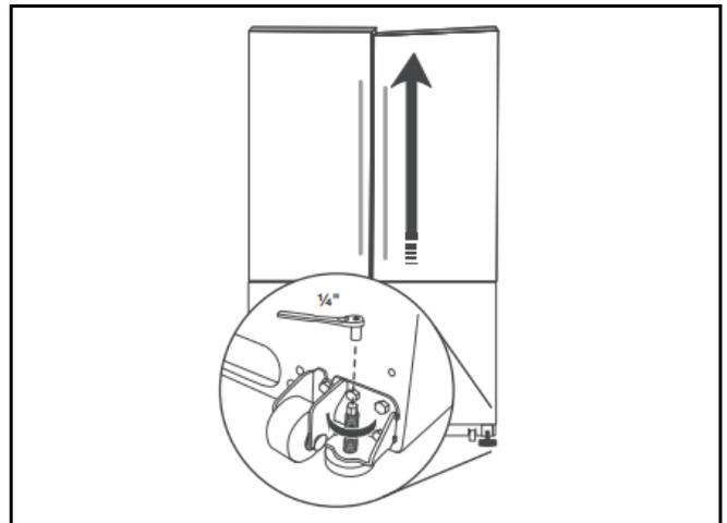
6. Make sure the refrigerator is steady. If the refrigerator seems unsteady or rolls forward when the door or drawer is opened adjust the leveling screws. Using a 1/4" hex driver, turn the leveling screw on each side clockwise until the rollers are up and the leveling feet are firmly against the floor.
