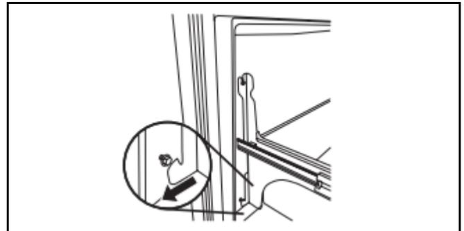
3. Completely tighten the four screws.
