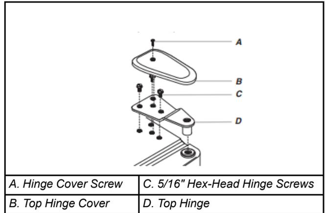
3. Adjust the door so that the bottom of the refrigerator door is aligned with the top of the freezer drawer. Tighten all screws.
