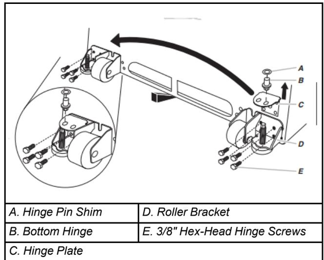
2. Remove the shim that you placed under the front edge of the refrigerator cabinet. Replace the freezer door.
