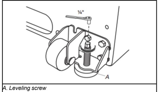
4. Open and close the doors to make sure they close as easily as you like. If not, increase the tilt by turning both leveling screws clockwise. It may take several turns of the leveling screw to allow the doors to close easier.
