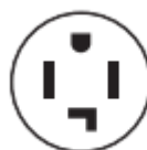
4-wire receptacle (14-30R)
